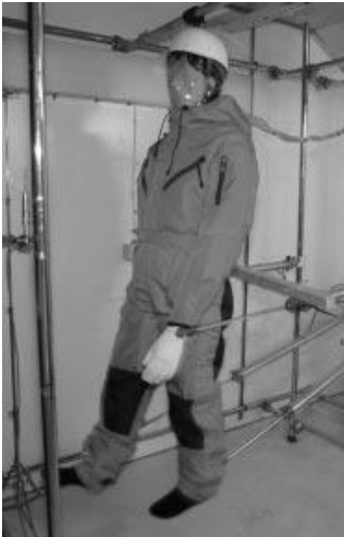
12.2 Walking thermal manikin for measurement of thermal insulation of clothing.
