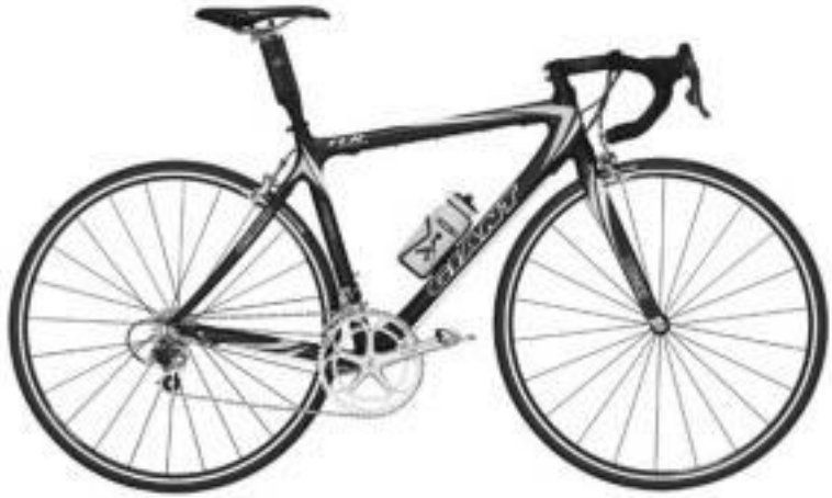
14.1 Lightweight race bicycle made of composite parts. (Source: http://www.giant-bicycles.com ).
