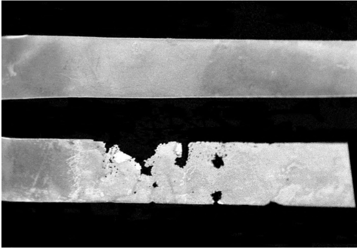
1.1 Biodegradation of poly(3-hydroxybutyrate) films under methanogenic conditions. The top strip was incubated in sterile medium and the bottom strip was incubated in anaerobic cultures for 10 days at 35°C. Initially, the strips were 0.016 mm thick and 1 cm × 7 cm. Reprinted with permission from Budwil [62]. Copyright 1995 K. Budwil.
