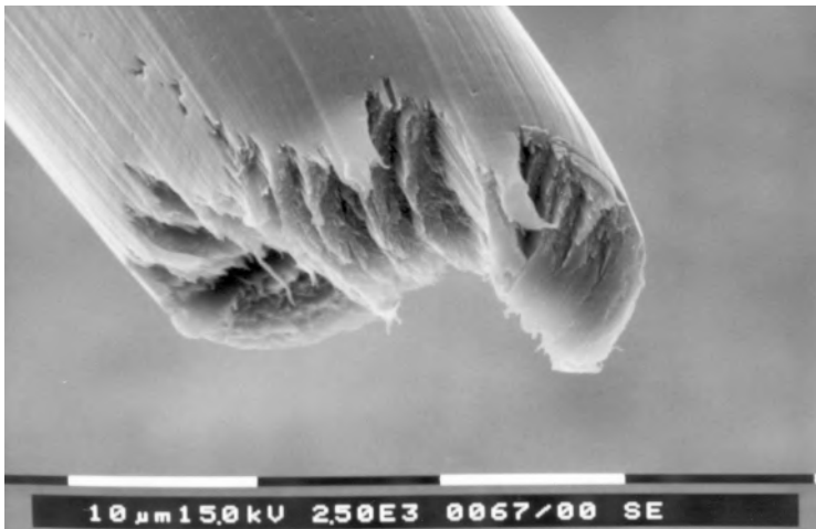
12.7 SEM micrograph showing the cross-section of fiber exhibiting the elongated fibrils. The fiber was obtained from spinning a 9% (w/w) cellulose solution at 30°C into methanol coagulant bath kept at -4°C with D_r above 2. Scale bar equals 10 \mu\text{m} .
