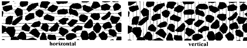
Figure 2. Determination of filament distances (chosen distance of cutting lines: 4 \mu\text{m} )
