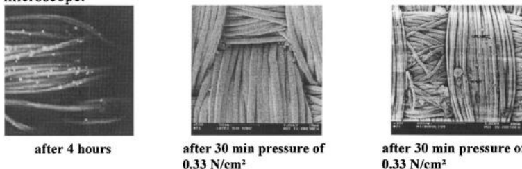
Figure 12. Micro spheres of 1 \mu\text{m} (left), latex micro spheres of 5 \mu\text{m} (centre) and micro polish particles of 3 \mu\text{m} (right) on the back of the fabric after penetration
