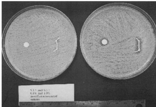
Fig. 1: Zones of inhibition for 0.1% moxifloxacin (left) and 1.0% moxifloxacin (right) coated sutures after 1 day in PBS buffer. For each plate the 1 cm suture fragment was on the right and the aliquot of exposed PBS buffer was spotted in the left.
