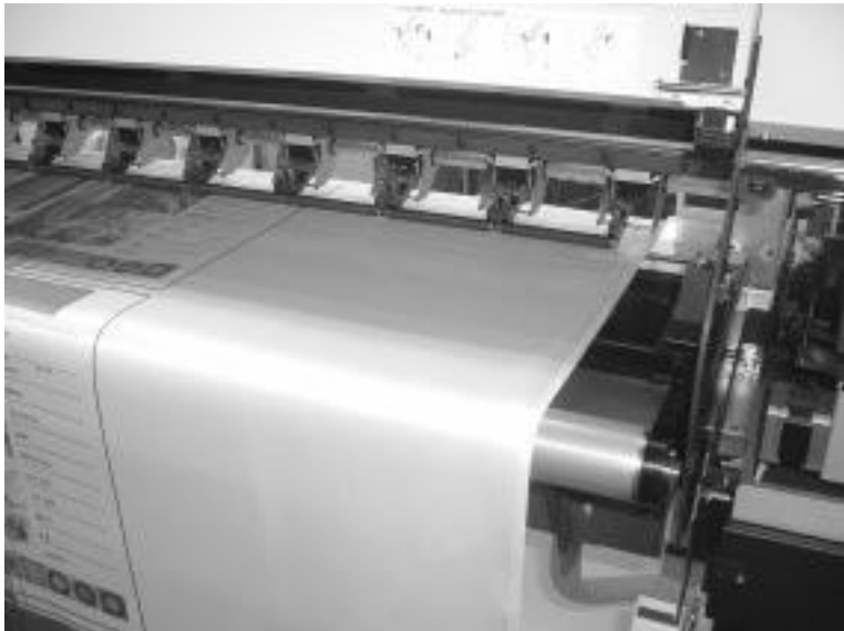
7.9 Tx2 fabric tension mechanism.
