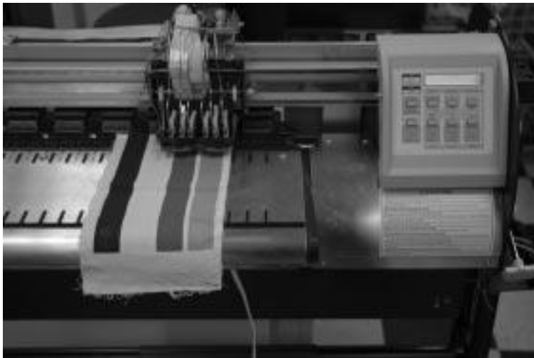
8.3 Printing plain weave cotton fabric with color stripes on Mutoh inkjet printer.
