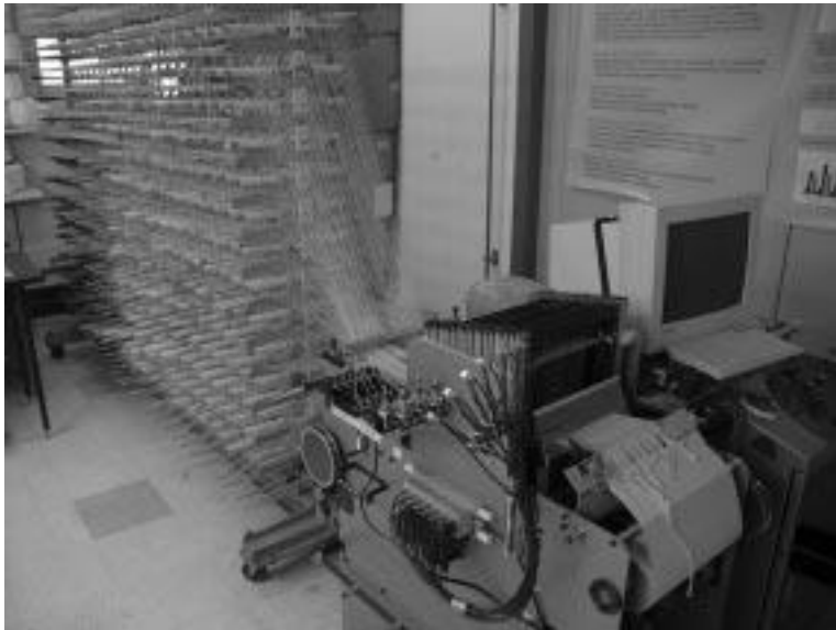
8.2 Weaving cotton fabric on a Sumagh 400 end sample loom.
