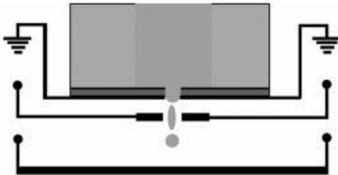
3.22 Drop-on-demand electro-hydrodynamic extraction ink jet.
