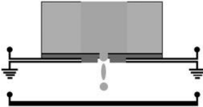
3.23 Drop-on-demand surface tension driven ink jet.
