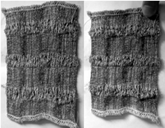
10.6 Shape memory recovery of SMP composite loosely woven fabric at 50 °C with recovery time (a) 0 sec, (b) 30 sec.
