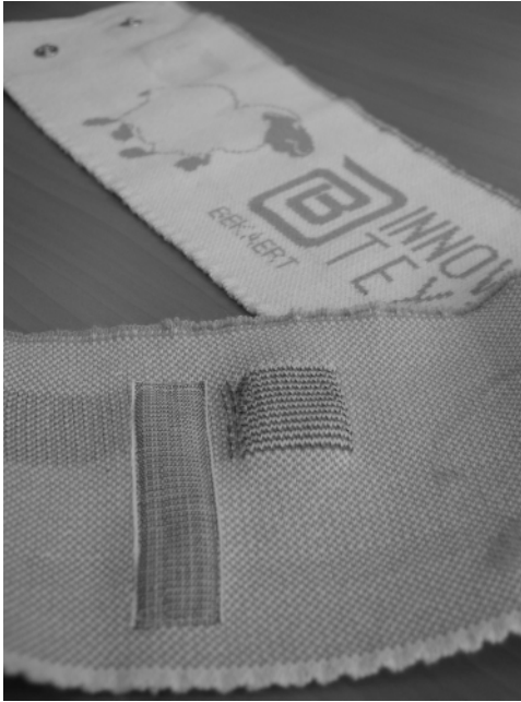
23.6 Belt with integrated sensors and interconnections.
