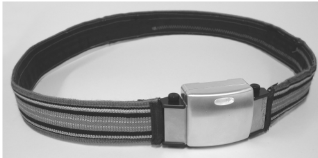
21.13 ETH-QBIC – a mobile computer (Xscale CPU, 256 MB SRAM, USB, RS-232, VGA, Bluetooth) integrated in a belt buckle; the belt houses the flexible batteries and interface connectors.
