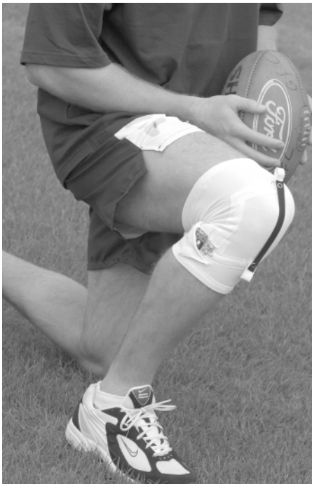
24.6 The Intelligent Knee Sleeve. The base sleeve is placed around the knee with the textile sensor placed over the kneecap (patella) and the electronics placed on the side of the sleeve hidden by a fabric pocket. Photo courtesy of CSIRO Textile and Fibre Technology.
