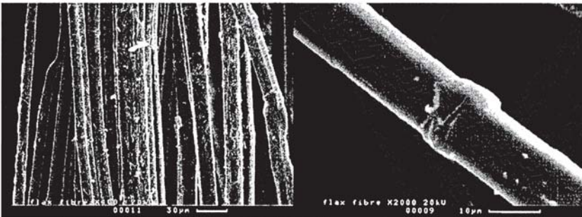
Figure 4. Flax fibre SEM
