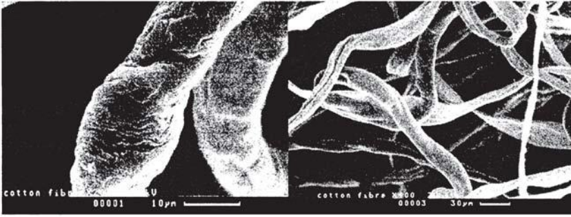
Figure 2. Cotton fibre SEM
