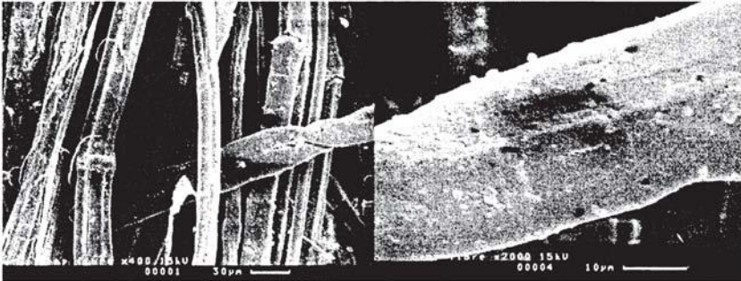
Figure 3. Hemp fibre SEM
