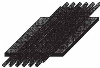
Figure 4: Fiber Lay-ups of 50/50 Combined Kenaf for Longitudinal and Transverse Composite
