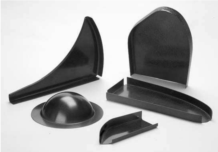
10.11 Prepreg preform shapes formed at CRC-ACS (clockwise from top left): a DDF rudder leading-edge rib with a concave flange; a DDF section of a rudder closure rib; a DDF flap leading-edge rib; a DDF rudder leading edge rib; a flanged dome shape formed using a rubber male punch and a metal female die with blank holder.
