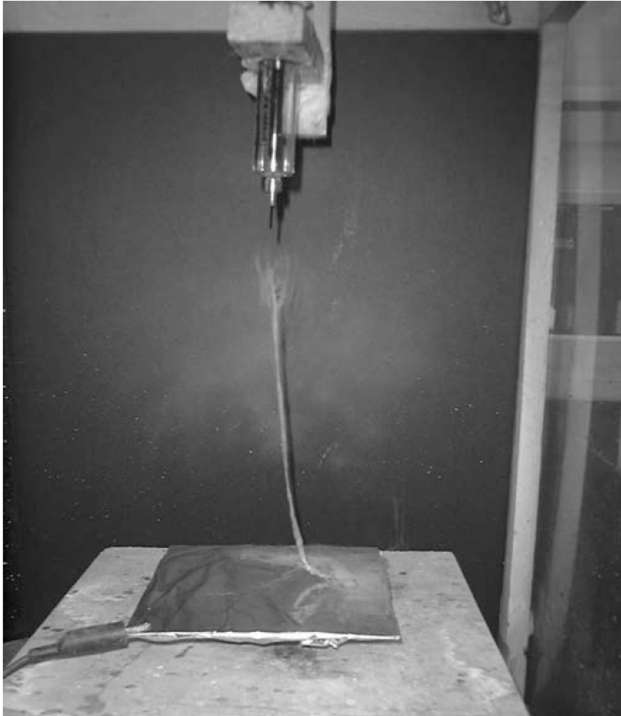
3.8 Self-assembled yarn formation. Reprinted with permission from reference 19 with kind permission from the author.
