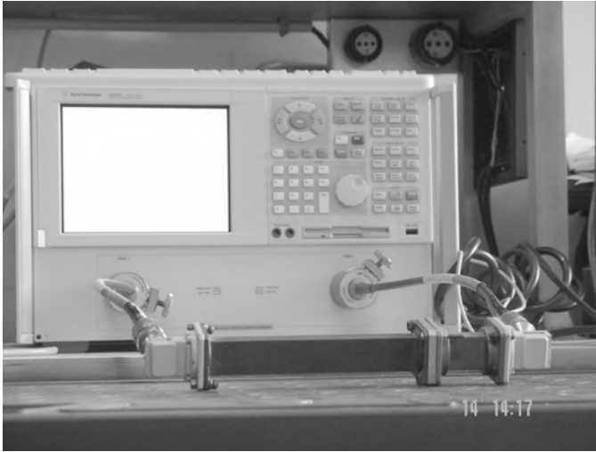
6.46 Agilent portable network analyzer (PNA) E8363B – experimental set-up. 64
