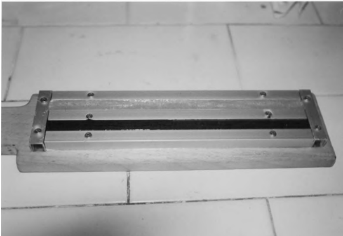
6.35 Nanostructured polymeric composite specimen for mechanical tests. 58
