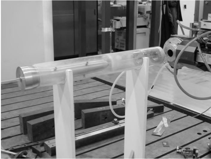
6.13 Laser ablation CO 2 apparatus for carbon nanotube synthesis. 55
