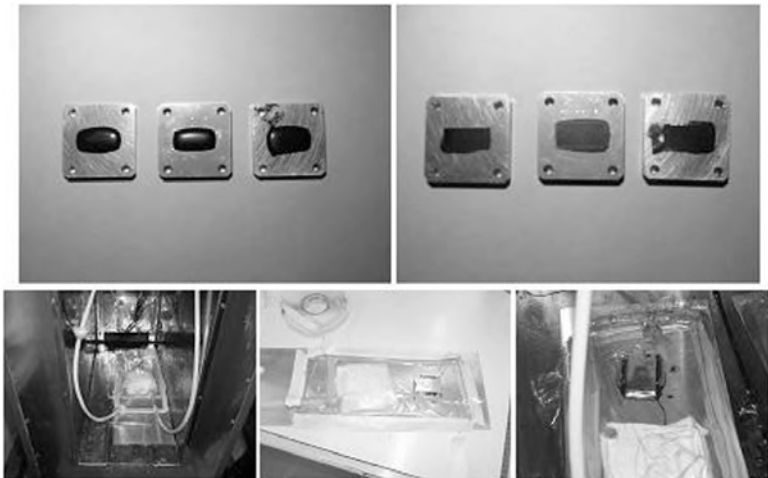
6.45 Nanostructured FSS samples (before the final mechanical removal of the residual material on the waveguide surfaces) and the relative manufacturing procedures. 64
