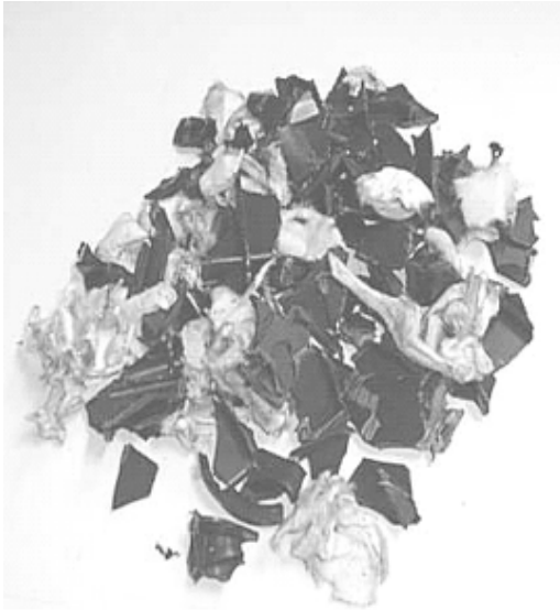
5.8 Crushing material of blocked filter.
