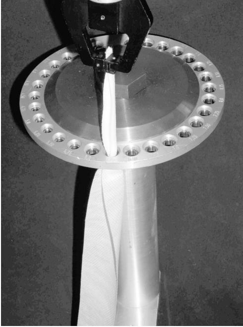
3.1 Pulling-through resistance device with different ring diameters.
