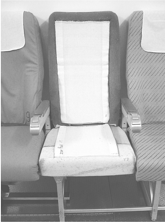
8.11 Modification of an aeroplane seat by means of a spacer fabric (Bartels, 2003).
