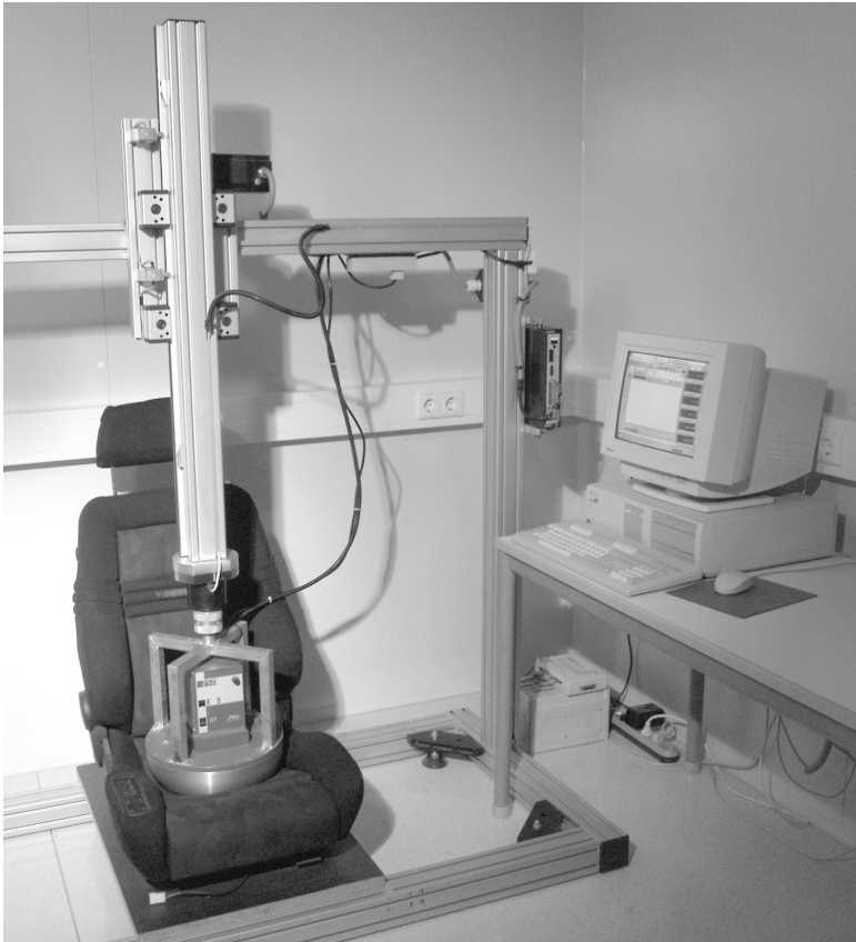
8.8 Photo of the seat comfort tester (upholstery tester) for testing the thermal properties of entire car seats.
