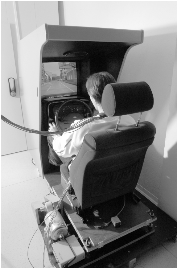
8.5 Seat trial with a human test subject on a driving simulator in a climatic chamber.
