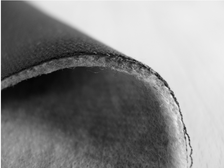
7.3 Three-dimensional stitch-bonded nonwoven type CALIWEB® laminated with cover fabric.
