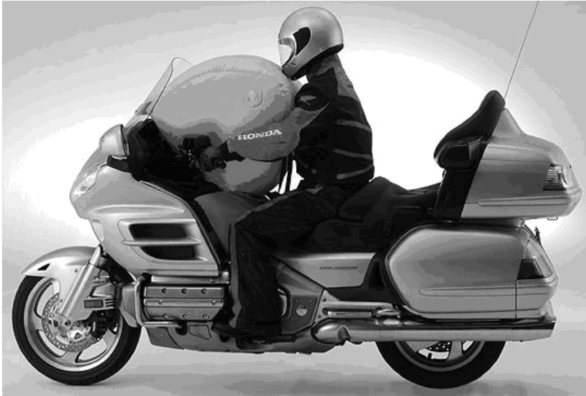
12.5 Airbag as a passive safety device for motorcycle. Courtesy: Honda marketing literature, 2006.
