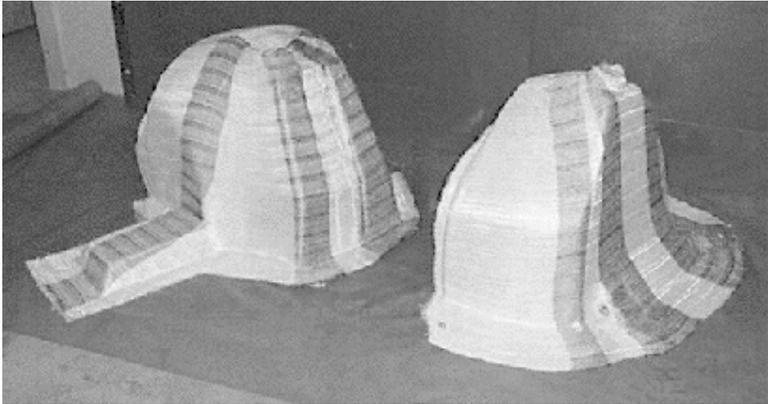
15.13 Picture of finished rear and front wheel well preforms, with near net-shape knitted fabrics encapsulating cap and mount sub-preforms. The black strips are selective carbon yarn laid-in according to structural requirements.
