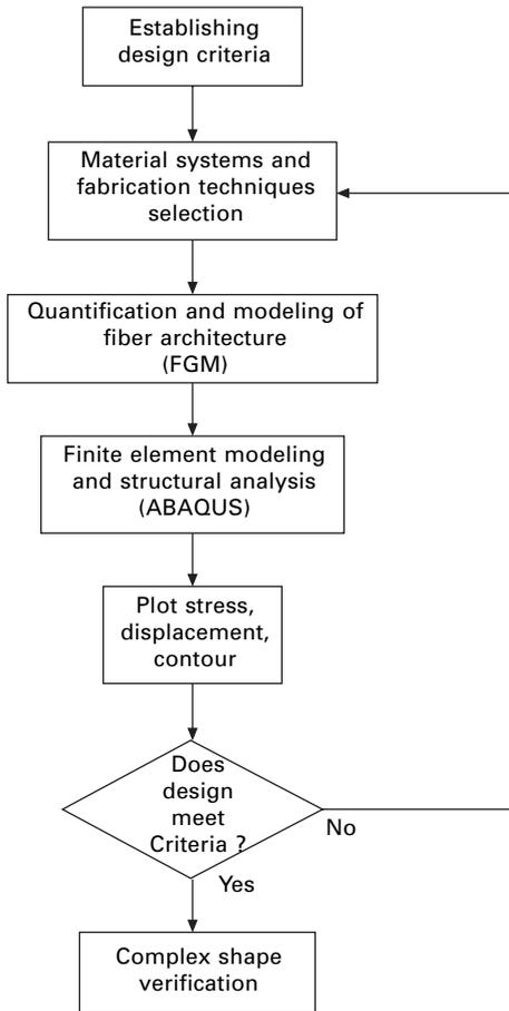
15.6 Logic flow of the integrated design for manufacturing methodology.
