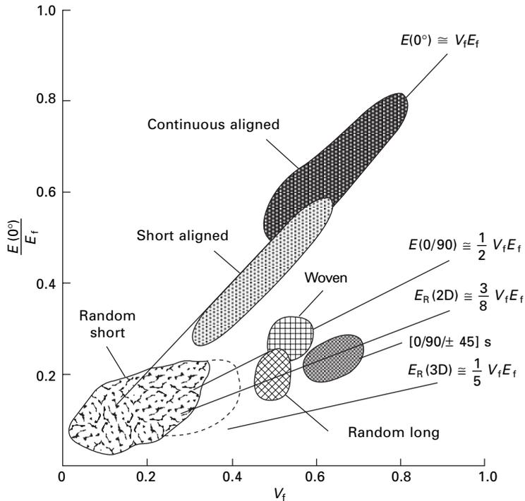
15.4 Fiber property translation efficiency as a function of fiber architecture and fiber volume fraction.
