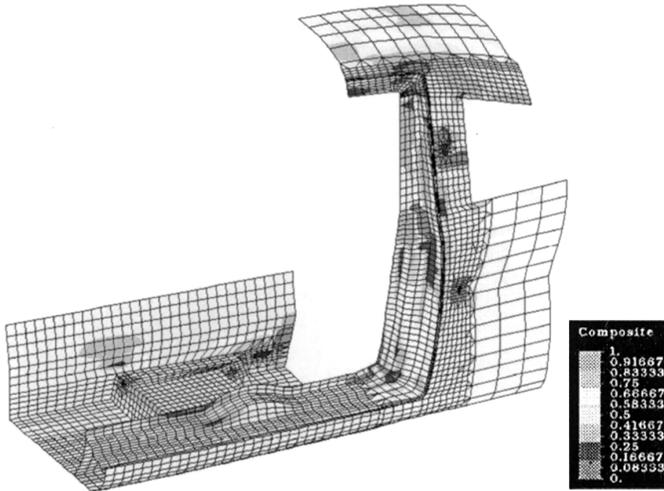
15.8 Finite element analysis of the B-pillar.
