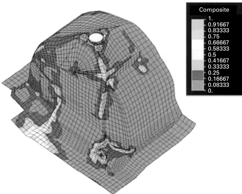
15.11 Finite element analysis of front wheel well with knitted reinforcement [17].
