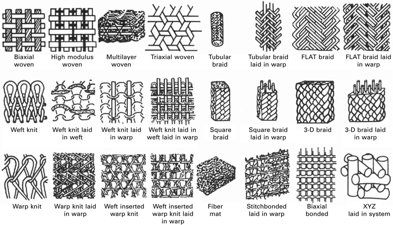
15.1 Textile structures for composite reinforcements.
