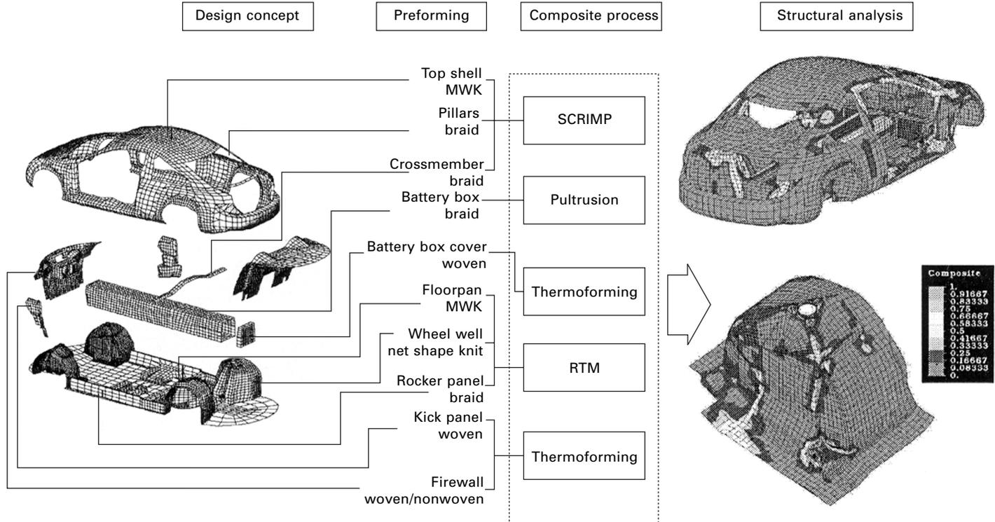
15.5 Composite parts breakdown of Sunrise™ BIW according to textile preforming processes and composite manufacturing processes.
