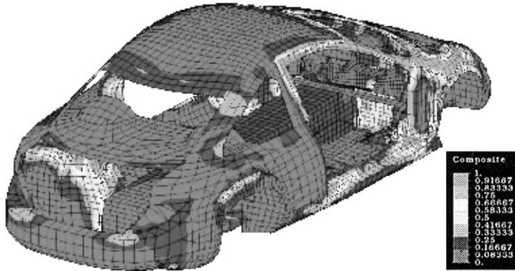
15.7 Stress contour from body torsion finite element analysis [16].
