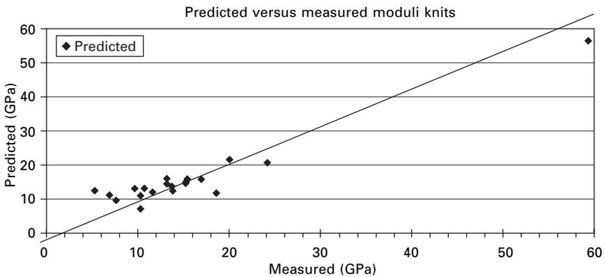
15.14 Predicted and experimental tensile moduli of the knitted composite wheel well.
