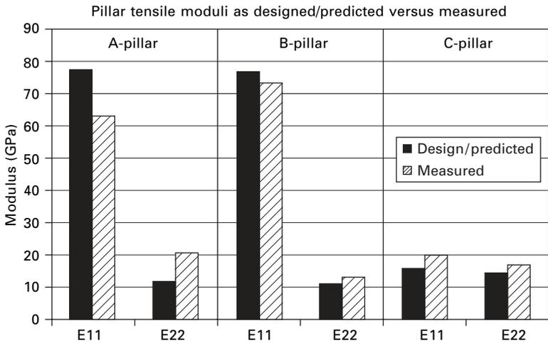
15.10 Comparison of the experimental and predicted moduli of the A, B, C pillars.
