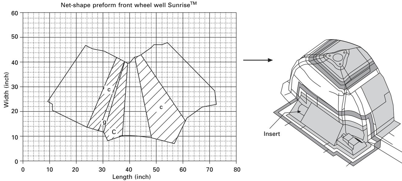
15.12 Net-shape 2D knitted preform for the front wheel wells; the fabric drapes around the mold easily produce the complex shaped part; the UD carbon reinforcements are integrated strategically into the preform during the knitting process.
