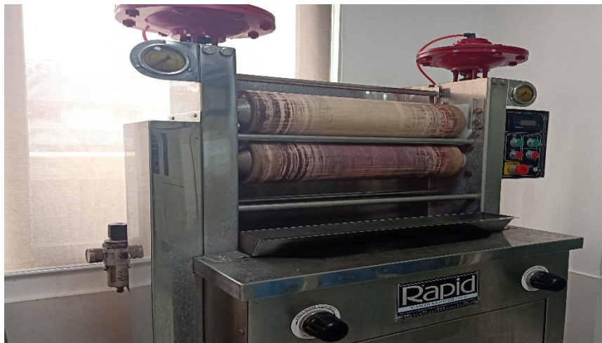
Figure 1. Cold pad batch lab dyeing machine
