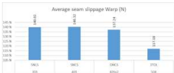
Figure 10: Comparative study on seam slippage (warp) based on stitch type
