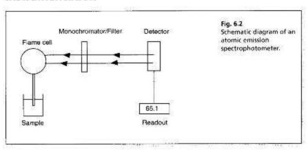
An atomic emission spectrophotometer (Fig. 6.2) is composed of the following components:
