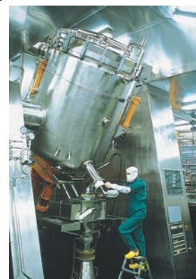
An industrial-scale reactor for preparation of an antibiotic.
