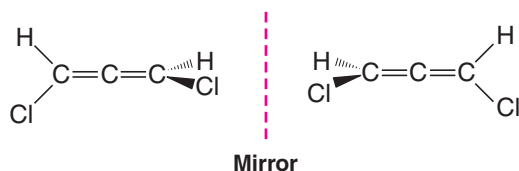
FIGURE 5.22 Enantiomeric forms of 1,3-dichloroallene. These two molecules are nonsuperposable mirror images of each other and are therefore chiral. They do not possess a tetrahedral atom with four different groups, however.
