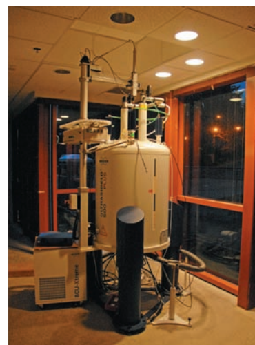
The superconducting magnet of an FTNMR spectrometer.
