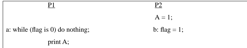
Figure 2-14 Point-to-point event synchronization using flags.
