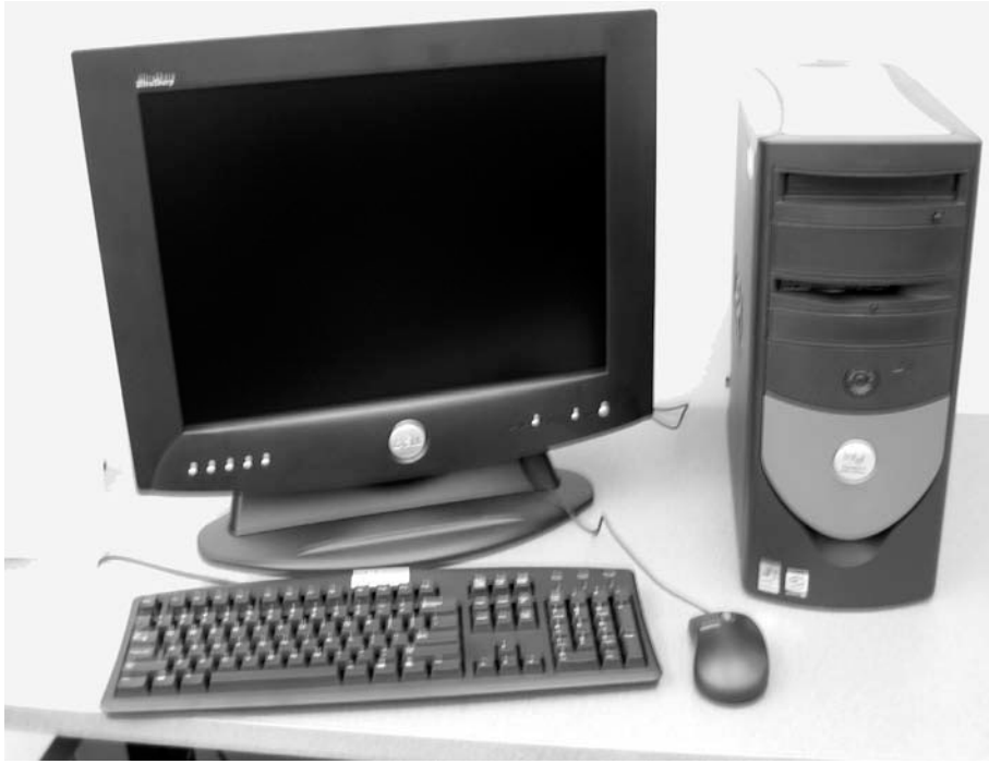
FIGURE 1.6 A desktop computer. The liquid crystal display (LCD) screen is the primary output device, and the keyboard and mouse are the primary input devices. The box contains the processor as well as additional I/O devices. This system is a Dell Optiplex GX260.
