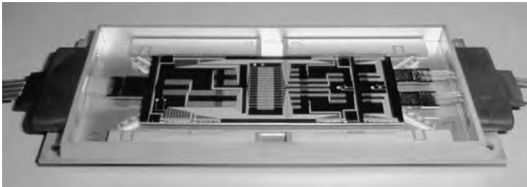
Figure 11.26 Chip architecture for an 8 \times 8 intelligent optical switching matrix with single-mode fiber: (a) structure block schematic; (b) OEIC module package [Ref. 86]
