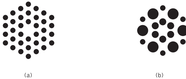
Figure 2.37 Two index-guided photonic crystal fiber structures. The dark areas are air holes while the white areas are silica
