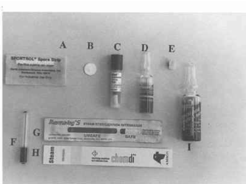
Fig. 23.1 Examples of biological and chemical indicators used for monitoring sterilization processes. (A and B) A spore strip (in a glassine envelope) and a spore disc, respectively; the spores are dried onto absorbent paper or fabric. (C) Attest™ indicator comprising a plastic vial containing a spore strip together with a sealed glass ampoule of culture medium; the ampoule is crushed after exposure and the medium immerses the strip. (D) Chemspor™ indicator in which bacterial spores are suspended in culture medium; the horizontal band on the ampoule also darkens on autoclaving to enable steam-exposed and non-exposed ampoules to be distinguished. (E) Plastic carrier with dried Bacillus stearothermophilus spores designed for monitoring low-temperature steam and formaldehyde cycles. (F) Browne's tube™; the liquid within the tube changes colour on heat exposure. (G) Thermalog™ strip in which a blue dye progresses from left to right during heat exposure. (H) Chemdi™ displays colour change in arrowed section of the strip after heating. (I) Chemspor™ which is a combined chemical and biological indicator; the ampoule contains a spore suspension in culture medium together with a second, smaller ampoule which contains a chemical indicator.
