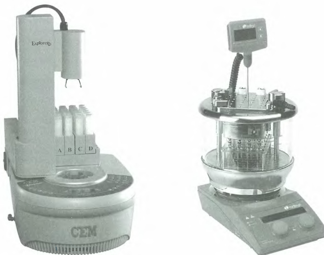
FIGURE 16.26 Laboratory stations for microwave assisted organic reactions. CEM Explorer-24, kindly supplied by CEM Corporation, NC (left).
