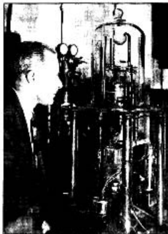
Walter Houser Brattain (1902–1987), one of the inventors of the transistor, looking at a vacuum evaporator used for depositing metal film electrodes on semiconductors (1937).
