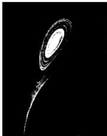
(e) Diffraction pattern produced by 40 keV electrons passing through zinc oxide powder. The distortion of the pattern was produced by a small magnet placed between the sample and the photographic plate. An X-ray diffraction pattern would not be affected by a magnetic field.
