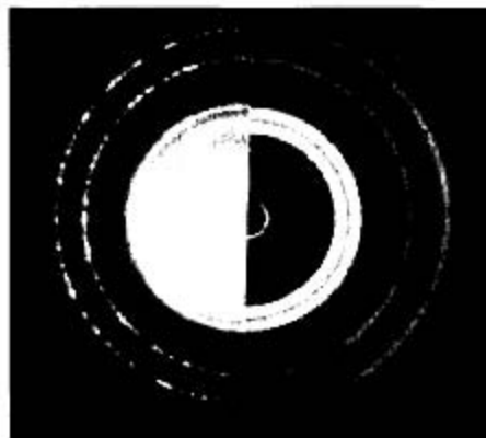
(d) Composite photograph showing diffraction patterns produced with an aluminum foil by X-rays and electrons of similar wavelength. Left: X-rays of \lambda = 0.071 nm. Right: Electrons of energy 600 eV.
