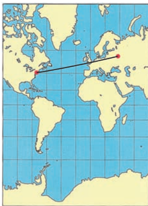
▲ Figure 7.3.2 A flight path with constant compass heading from New York City to Moscow follows a spiral toward the North Pole but is a straight line segment on a Mercator projection.
