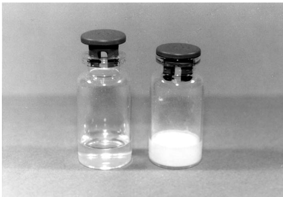
Fig. 3 Vials typically used for lyophilization showing slotted stopper in the open and closed positions.
