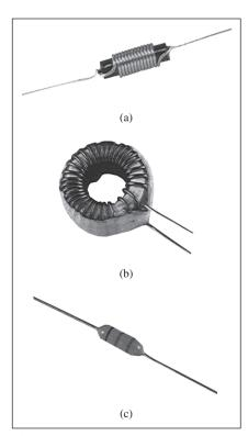
**Figure 6.22**Various types of inductors: (a) solenoidal wound inductor, (b) toroidal inductor, (c) chip inductor.
