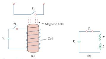
**Figure 7.77** A relay circuit.
