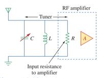
**Figure 14.63** The tuner circuit for Example 14.17.
