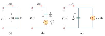
**Figure 16.2** Representation of a capacitor: (a) time-domain, (b,c) *s*-domain equivalents.
