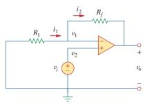
**Figure 5.16**The noninverting amplifier.
