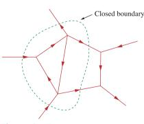
**Figure 2.17** Applying KCL to a closed boundary.
