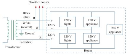
**Figure 12.38**Single-phase three-wire residential wiring.
