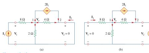
**Figure 19.18** Solution of Example 19.4: (a) finding  $y_{11}$  and  $y_{21}$ , (b) finding  $y_{12}$  and  $y_{22}$ .
