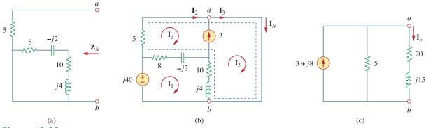
Figure 10.29 Solution of the circuit in Fig. 10.28: (a) finding  $\mathbf{Z}_N$ , (b) finding  $\mathbf{V}_N$ , (c) calculating  $\mathbf{I}_O$ .
