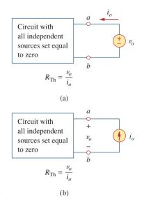
**Figure 4.25** Finding  $R_{\text{Th}}$  when circuit has dependent sources.
