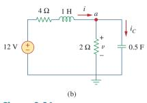
**Figure 8.26** Equivalent circuit of the circuit in Fig. 8.25 for: (a) t < 0, (b) t > 0.
