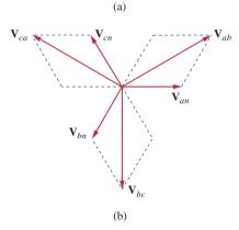
**Figure 12.11**Phasor diagrams illustrating the relationship between line voltages and phase voltages.
