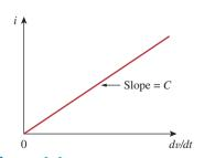
**Figure 6.6**Current-voltage relationship of a capacitor.
