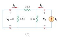
**Figure 19.15** For Example 19.3: (a) finding  $\mathbf{y}_{11}$  and  $\mathbf{y}_{21}$ , (b) finding  $\mathbf{y}_{12}$  and  $\mathbf{y}_{22}$ .
