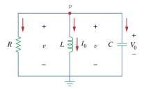
**Figure 8.13** A source-free parallel *RLC* circuit.
