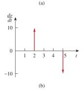
**Figure 7.32** (a) Decomposition of the pulse in Fig. 7.31, (b) derivative of the pulse in Fig. 7.31.
