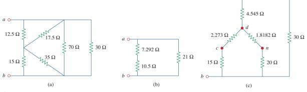
**Figure 2.53** Equivalent circuits to Fig. 2.52, with the voltage source removed.
