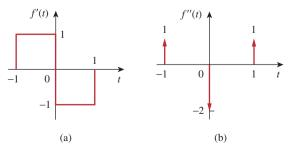
**Figure 18.15** First and second derivatives of f(t) in Fig. 18.14; for Example 18.5.
