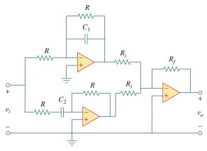
**Figure 14.47** Active bandreject filter.
