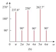
**Figure 17.8** For Example 17.2: (a) amplitude spectrum, (b) phase spectrum.
