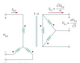
**Figure 13.48** Y- $\Delta$  three-phase transformer connection.
