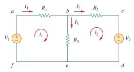
**Figure 3.17** A circuit with two meshes.
