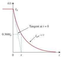
**Figure 7.12** The current response of the *RL* circuit.
