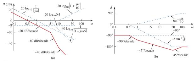
**Figure 14.15**Bode plots for Example 14.4: (a) magnitude plot, (b) phase plot.
