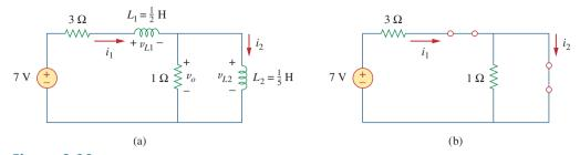
**Figure 8.30** Equivalent circuit of that in Fig. 8.29 for: (a) t > 0, (b)  $t \to \infty$ .
