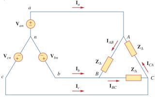
Figure 12.14 Balanced Y- $\Delta$  connection.
