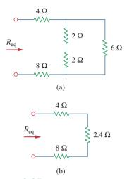
**Figure 2.35** Equivalent circuits for Example 2.9.
