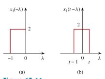
**Figure 15.11** (a) Folding  $x_1(\lambda)$ , (b) shifting  $x_1(-\lambda)$  by t.
