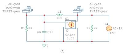
**Figure 19.53** For Example 19.16: (a) circuit for determining  $\mathbf{z}_{11}$  and  $\mathbf{z}_{21}$ , (b) circuit for determining  $\mathbf{z}_{12}$  and  $\mathbf{z}_{22}$ .
