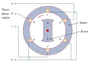
**Figure 12.4** A three-phase generator.
