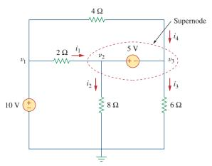
**Figure 3.7** A circuit with a supernode.
