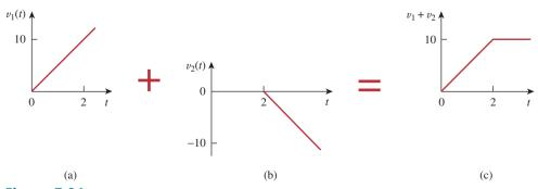
**Figure 7.36** Partial decomposition of v(t) in Fig. 7.35.
