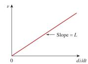
Figure 6.24 Voltage-current relationship of an inductor.
