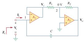
**Figure 10.41**Capacitance multiplier.
