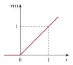
**Figure 7.29** The unit ramp function.
