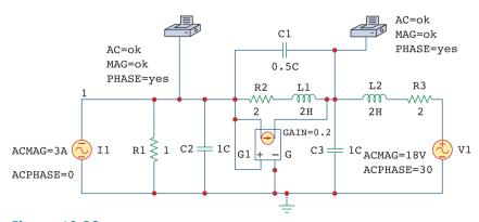
**Figure 10.39** Schematic for the circuit in the Fig. 10.38.
