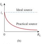
**Figure 4.60** (a) Practical current source connected to a load  $R_L$ , (b) load current decreases as  $R_L$  increases.
