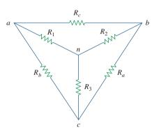
**Figure 2.49** Superposition of Y and  $\Delta$  networks as an aid in transforming one to the other.
