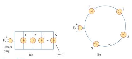
**Figure 2.55**(a) Parallel connection of light bulbs, (b) series connection of light bulbs.
