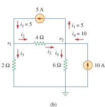
**Figure 3.3** For Example 3.1: (a) original circuit, (b) circuit for analysis.
