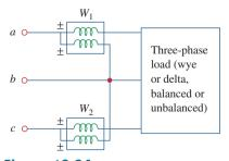
**Figure 12.34**Two-wattmeter method for measuring three-phase power.
