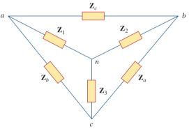
**Figure 9.22** Superimposed *Y* and  $\Delta$  networks.
