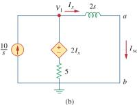
**Figure 16.15** For Example 16.6: (a) finding  $V_{\text{Th}}$ , (b) determining  $Z_{\text{Th}}$ .
