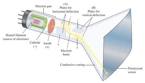
**Figure 1.17** Cathode-ray tube.
