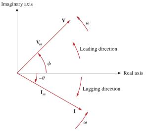
**Figure 9.8** A phasor diagram showing  $\mathbf{V} = V_m / \phi$  and  $\mathbf{I} = I_m / -\theta$ .
