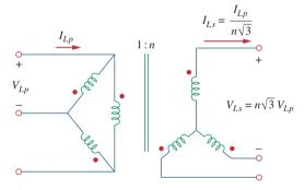
Figure 13.49  $\Delta$ -Y three-phase transformer connection.
