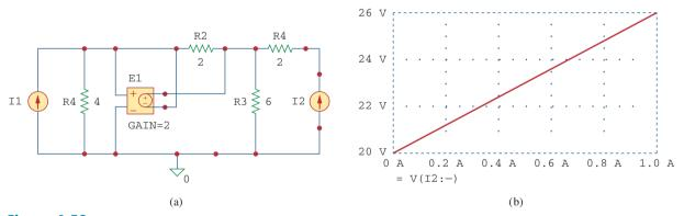
**Figure 4.53** For Example 4.14: (a) schematic and (b) plot for finding  $R_{\rm Th}$  and  $V_{\rm Th}$ .
