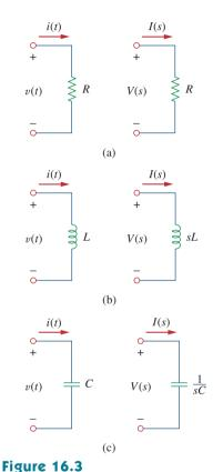
Time-domain and *s*-domain representations of passive elements under zero initial conditions.
