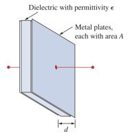
**Figure 6.1** A typical capacitor.
