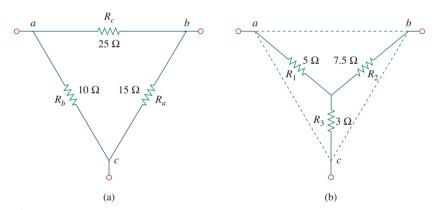
**Figure 2.50** For Example 2.14: (a) original  $\Delta$  network, (b) Y equivalent network.
