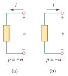
**Figure 1.8**Reference polarities for power using the passive sign convention: (a) absorbing
