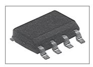
**Figure 5.1** A typical operational amplifier. Courtesy of Tech America.
