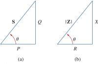
**Figure 11.21** (a) Power triangle, (b) impedance triangle.
