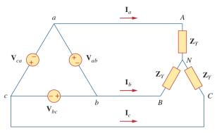
Figure 12.18 A balanced  $\Delta$ -Y connection.
