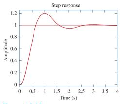
Figure 14.60 The Step response of  $H(s) = \frac{12}{(s^2 + 3s + 12)}$ .
