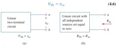
**Figure 4.24** Finding  $V_{\text{Th}}$  and  $R_{\text{Th}}$ .
