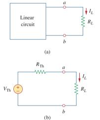
**Figure 4.26** A circuit with a load: (a) original circuit, (b) Thevenin equivalent.
