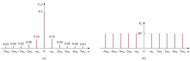
**Figure 17.31** For Example 17.11: (a) amplitude spectrum, (b) phase spectrum.
