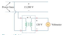
**Figure 13.61** A transformer providing isolation between the power lines and the voltmeter.
