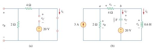
**Figure 8.6** The circuit in Fig. 8.5 for: (a)  $t = 0^-$ , (b)  $t = 0^+$ .
