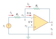
**Figure 5.10** The inverting amplifier.
