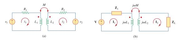
**Figure 13.7**Time-domain analysis of a circuit containing coupled coils (a) and frequency-domain analysis of a circuit containing coupled coils (b).
