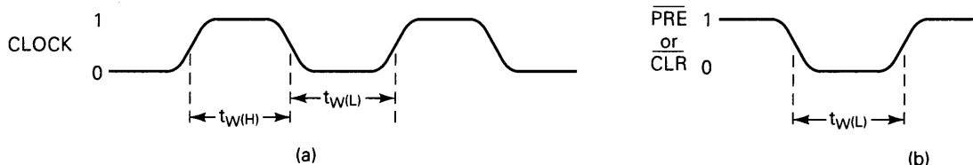
FIGURE 5-34 (a) Clock LOW and HIGH times; (b) asynchronous pulse width.
