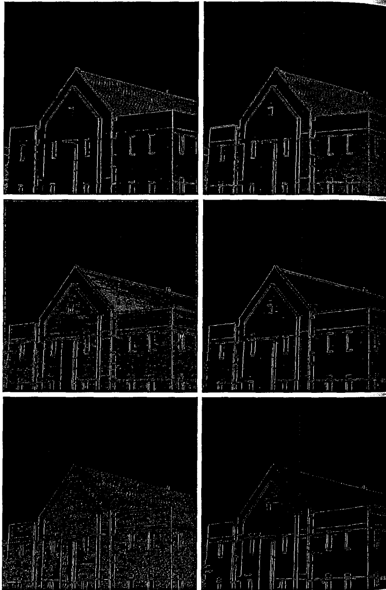
FIGURE 10.7 Left column: Default results for the Sobel, LoG, and Canny edge detectors. Right column: Results obtained interactively to bring out the principal features in the original image of Fig. 10.6(a) while reducing irrelevant, fine detail. The Canny edge detector produced the best results by far.
