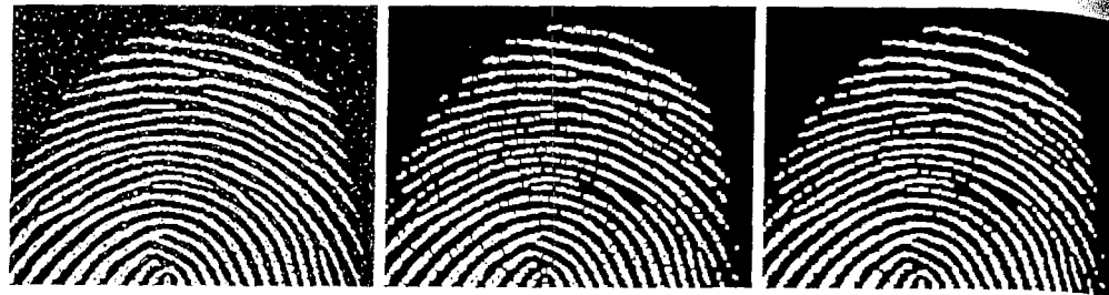
FIGURE 9.11 (a) Noisy fingerprint image. (b) Opening of image. (c) Opening followed by closing. (Original image courtesy of the National Institute of Standards and Technology.)
