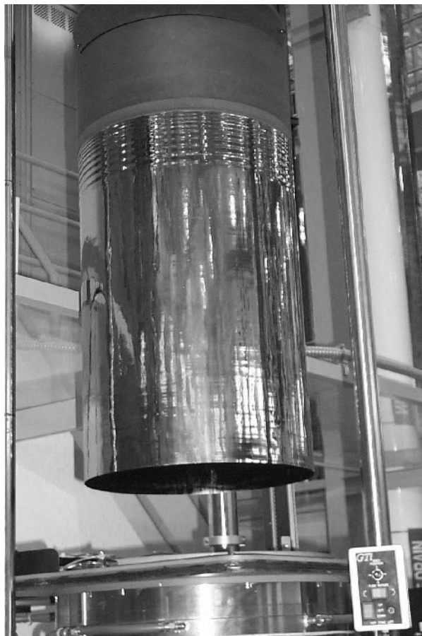
Figure 6.23 Experimental 50-cm-diameter EFG cylinder exiting from furnace
