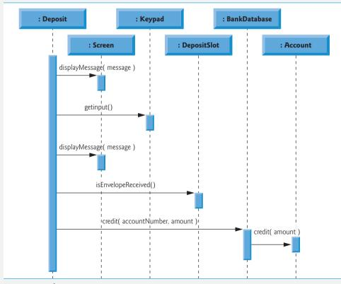
Fig. 25.30 Sequence diagram that models a Deposit executing.
