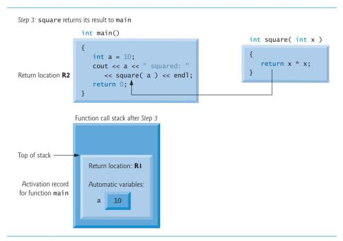
Fig. 6.16 Function call stack after function square returns to main.
