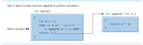
**Fig. 6.15** | Function call stack after main invokes square to perform the calculation. (Part 1 of 2.)
