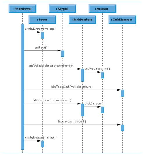
**Fig. 25.25** Sequence diagram that models a Withdrawal executing.
