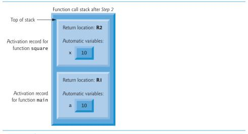
**Fig. 6.15** | Function call stack after main invokes square to perform the calculation. (Part 2 of 2.)
