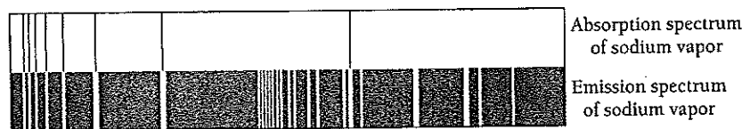
Figure 4.9 The dark lines in the absorption spectrum of an element correspond to bright lines in its emission spectrum.
