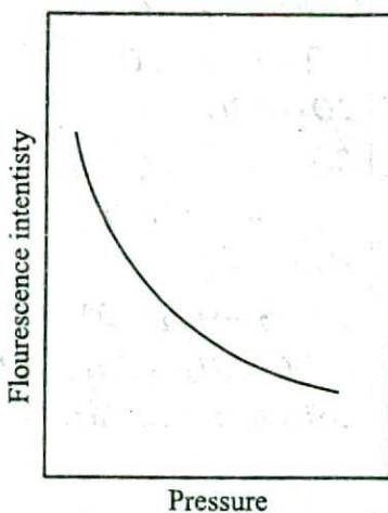
Figure 12.23 Fluorescence intensity of excited NO_2 plotted against pressure.
