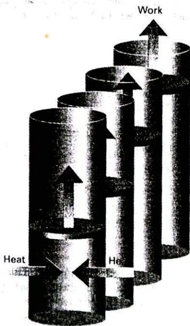
2.13 When a system is subjected to constant pressure and is free to change its volume, some of the energy supplied as heat may escape back into the surroundings as work. In such a case, the change in internal energy is smaller than the energy supplied as heat.
