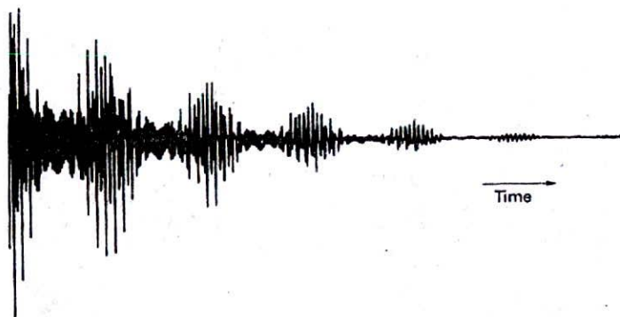
18.32 A free induction decay signal of a sample of ethanol. Its Fourier transform is the frequency-domain spectrum shown in Fig. 18.4.
