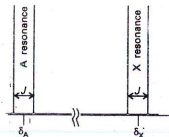
18.11 The effect of spin-spin coupling on an AX spectrum. Each resonance is split into two lines separated by J . The pairs of resonances are centred on the chemical shifts of the protons in the absence of spin-spin coupling.
