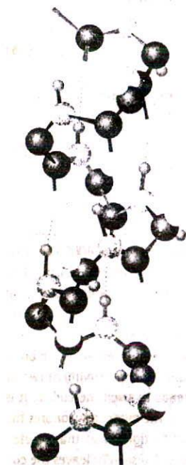
23.17 The dimensions that characterize the peptide link. The C—CO—NH—C atoms define a plane (the C—N bond has partial double-bond character), but there is rotational freedom around the C—CO and N—C bonds.
