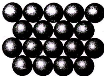
21.34 The first layer of close-packed spheres used to build a three-dimensional close-packed structure.
