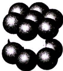
21.37 A fragment of the structure shown in Fig. 21.36 revealing the (a) hexagonal (b) cubic symmetry. The tints on the spheres are the same as for the layers in Fig. 21.36.
