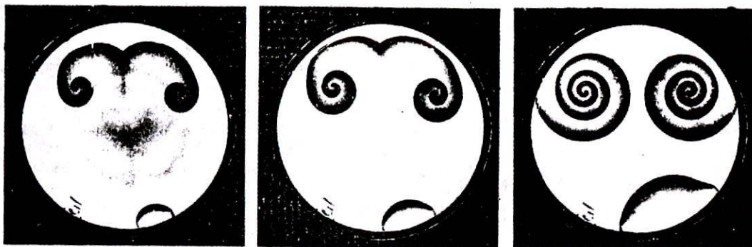
26.12 Some reactions show oscillations in time; some show spatially periodic variations. This sequence of photographs shows the emergence of a spatial pattern.
