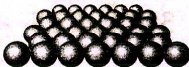
28.2 A schematic diagram of the flat surface of a solid. This primitive model is largely supported by surface-tunnelling microscope images (see Fig. 28.20).
