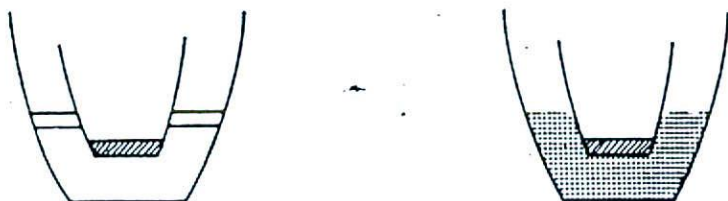
FIGURE 2.3: Crucible assemblies when igniting to constant weight; on left, asbestos ring support; on right, support by means of porcelain fragments.
