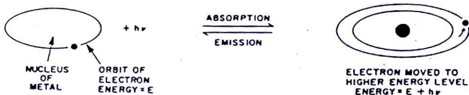
FIGURE 5.1: Relationship between atomic emission and atomic absorption.
