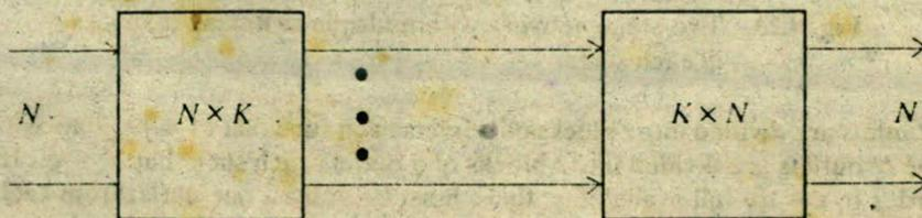
Fig. 4.22 A two-stage representation of an  $N \times N$  network.
