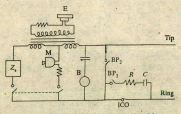
B = bell BP = by-pass switch ICO = impulsing contact
