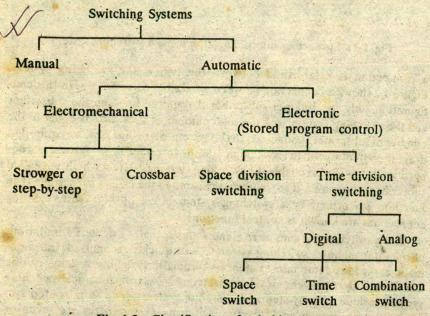
Fig. 1.3 Classification of switching systems.
