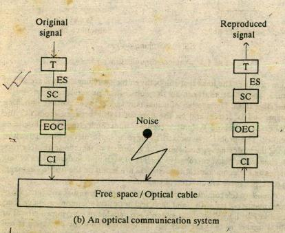
( CI = channel interface EOC = electrical to optical converter ES = electrical signal OEC = optical to electrical converter SC = signal conditioner T = transducer.
