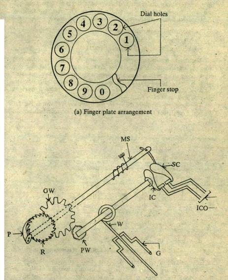
(b) Impulsing mechanism
