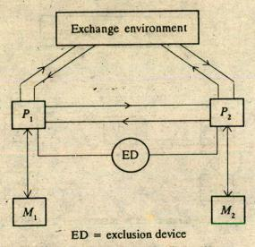
Fig. 4.6 Load sharing configuration.
