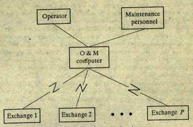
Fig. 4.10 Remote operation and maintenance.
