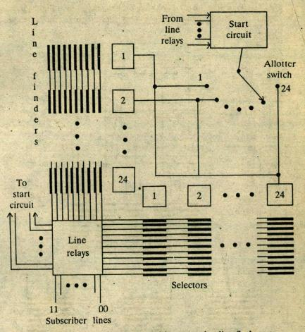
Fig. 2.12 100-line exchange with two-motion line finders.
