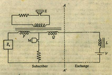
& Fig. 1.8 A telephone circuit with sidetone coupling.
