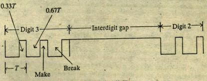
Fig. 2.1 Pulse dialling.
