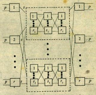
Fig. 4.27 Five-Stage switching network.
