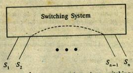
Fig. 1.2 Subscriber interconnection using a switching system.
