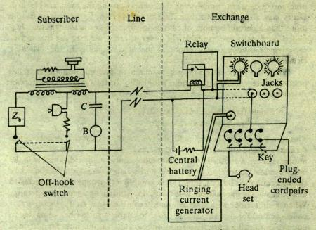
Fig. 1.11 Manned central battery exchange.
