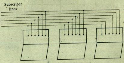
Fig. 1.13 Multitermination boards.
