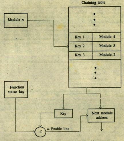
Fig. 4.16 Module chaining through table.
