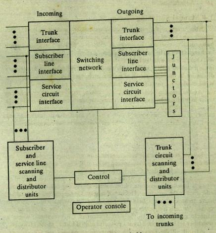
Fig. 1.10 Elements of a switching system.
