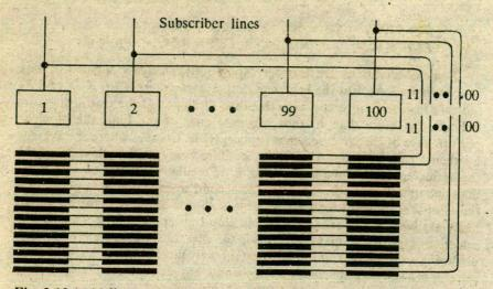
Fig. 2.10 100-line exchange with one two-motion selector per subscriber.
