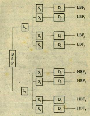
BSF = band separation filter D = detector HBF = high band frequency L = limiter LBF = low band frequency S = selector circuit
