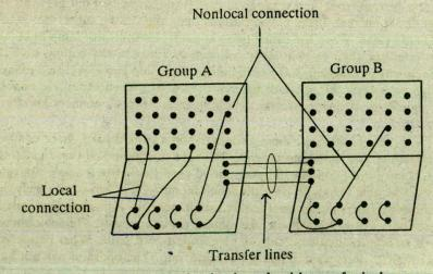
Fig. 1.12 Single termination boards with transfer jacks.
