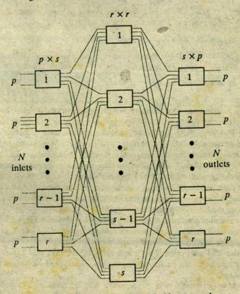
Fig. 4.24  $N \times N$  three-stage switching network.
