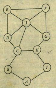
Fig. 3.1 A multiexchange network.
