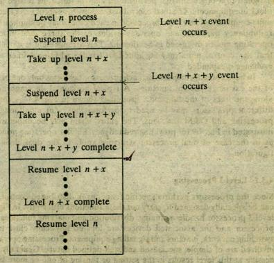
Fig. 4.8 Interrupt processing.
