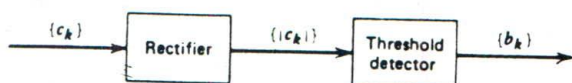
Figure 6.7 Detector for recovering original binary sequence from the precoded duobinary coder output.
