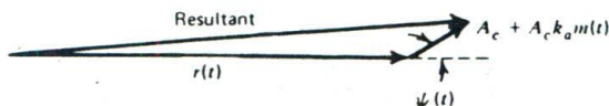
Figure 9.6 Phasor diagram for AM wave plus narrow-band noise for the case of low carrier-to-noise ratio.
